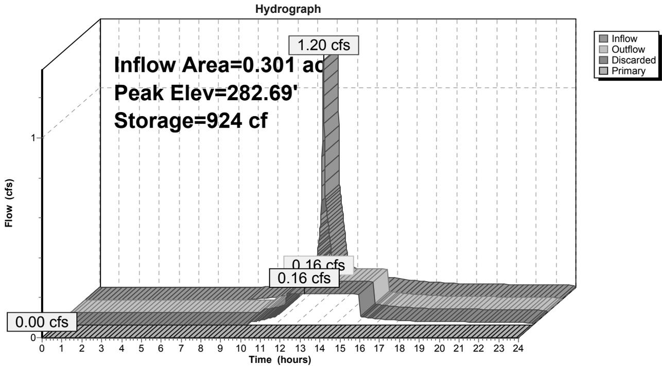
**Stage-Discharge for Pond PB6A: Porous Pavement**
